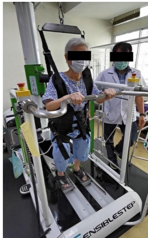
Figure 1. 'SensibleSTEP' Robotic gait training device
